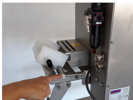
Image 5, Removing safety sensor
